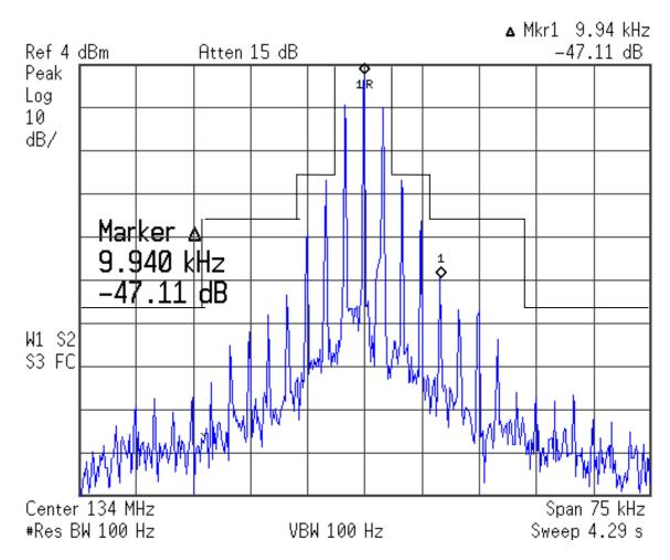
Measured emissions with spectral mask for 25 kHz channel spacing § 87.139 (b).
