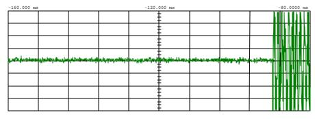
Trigger mode : Edge On Positive Edge Of Chan2 Trigger Level Chan2 = -175.000 mV (noise reject ON) Holdoff = 40.000 ns
