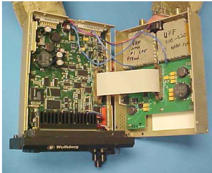
Unit Opened Showing Connection between Power Supply and CPU Board Ribbon Cable. Also Blue RF cables run from ITM module to Power Amp Modules.
