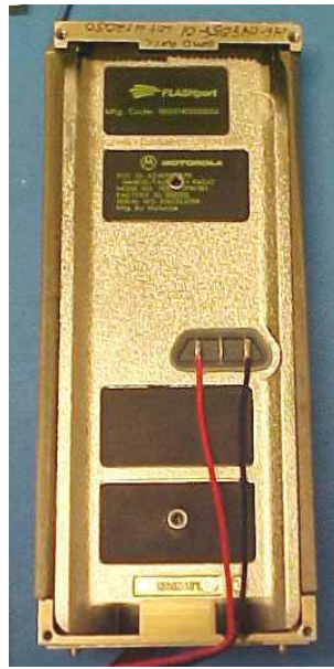
View of Power cables on underside of ITM
