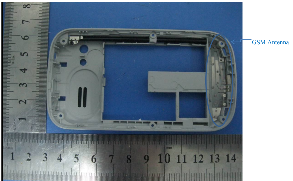
GSM Antenna - Top View
