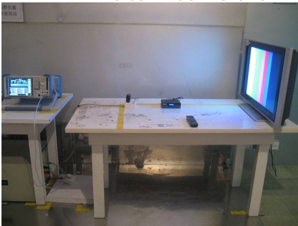
TEST SETUP OF CONDUCTED EMISSION (HDMI and AV output)
