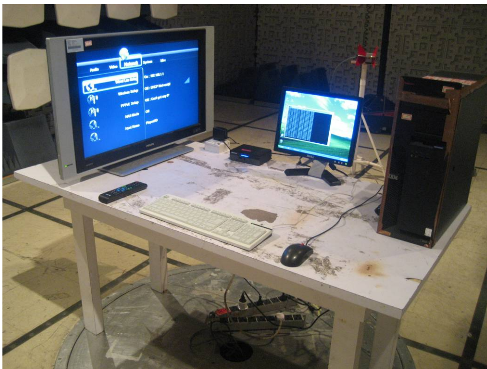
TEST SETUP OF RADIATED EMISSION (ABOVE 1 GHZ)
