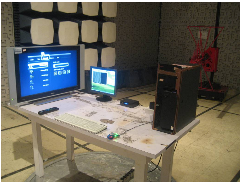
TEST SETUP OF RADIATED EMISSION (LAN)
