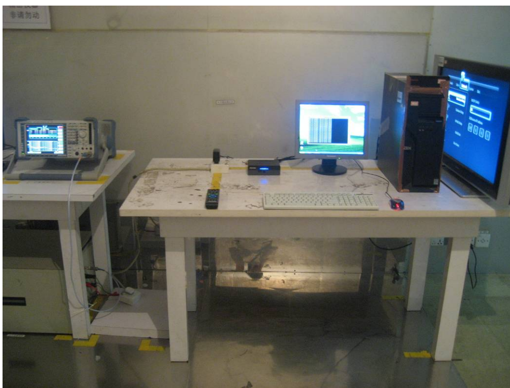
TEST SETUP OF CONDUCTED EMISSION (LAN )
