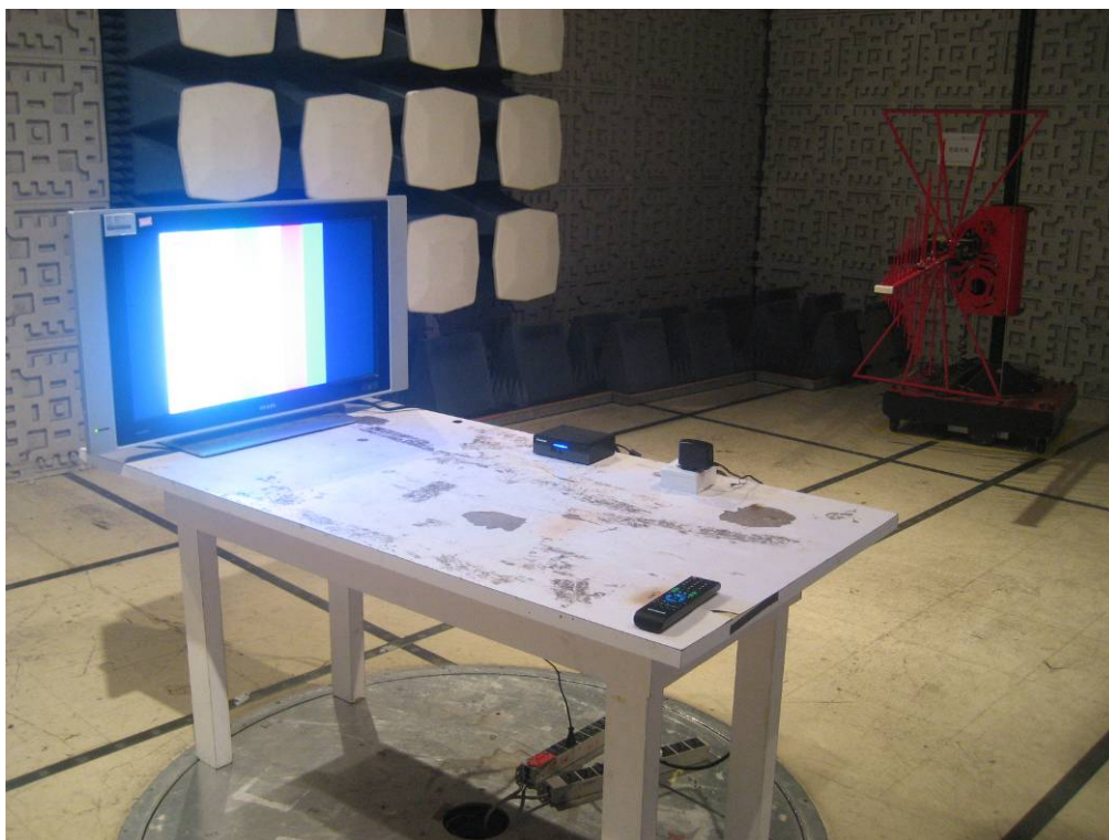
TEST SETUP OF RADIATED EMISSION (HDMI and AV output)
