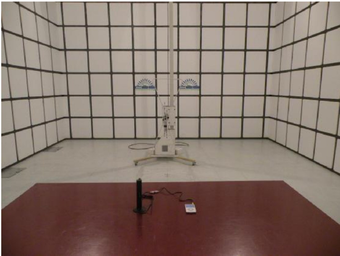
Radiated Emission Test Setup in Chamber
