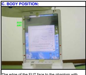
The edge of the EUT face to the phantom with 0mm-separation distance.
