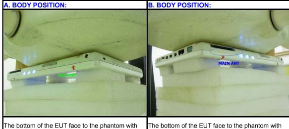
The bottom of the EUT face to the phantom with 0mm-separation distance. The bottom of the EUT face to the phantom with 0mm-separation distance.
