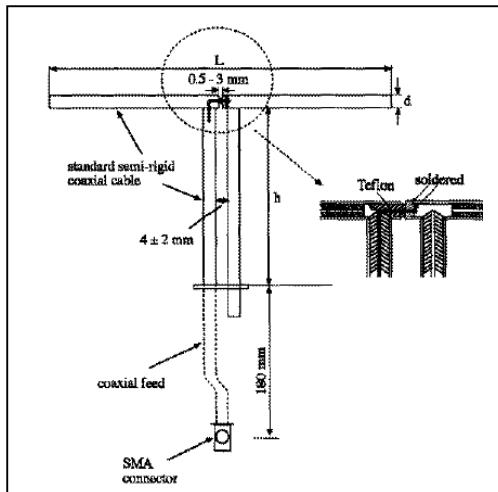
The dipoles used is based on the IEEE-1528 standard, and is complied with mechanical and electrical specifications in line with the requirements of both IEEE and FCC Supplement C. the table below provides details for the mechanical and electrical specifications for the dipoles.
