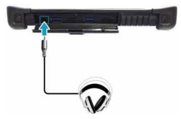
❖ To connect to a microphone, open the I/O port cover and plug the microphone cable into the audio combo of your device.
