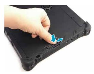
2. Remove the battery out of the battery compartment.
