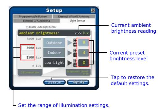
To setup the light sensor settings, do the following:
