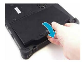
3. Slide the battery latch to the lock position to secure the battery.
