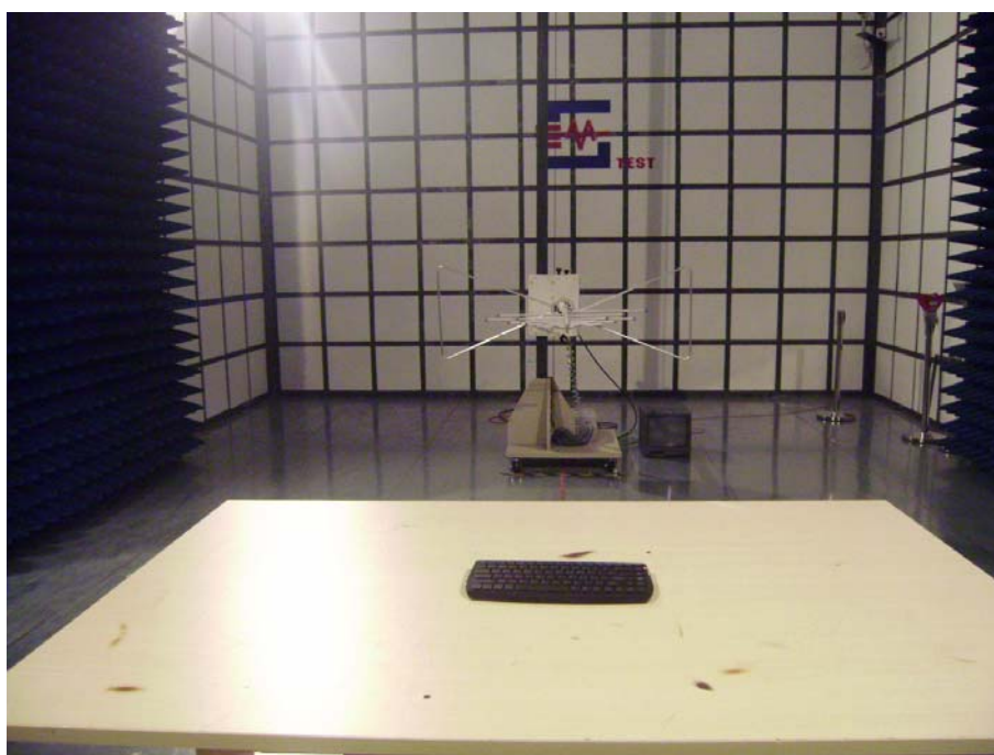
Radiation Emission Test Setup (30MHz to 1GHz)
