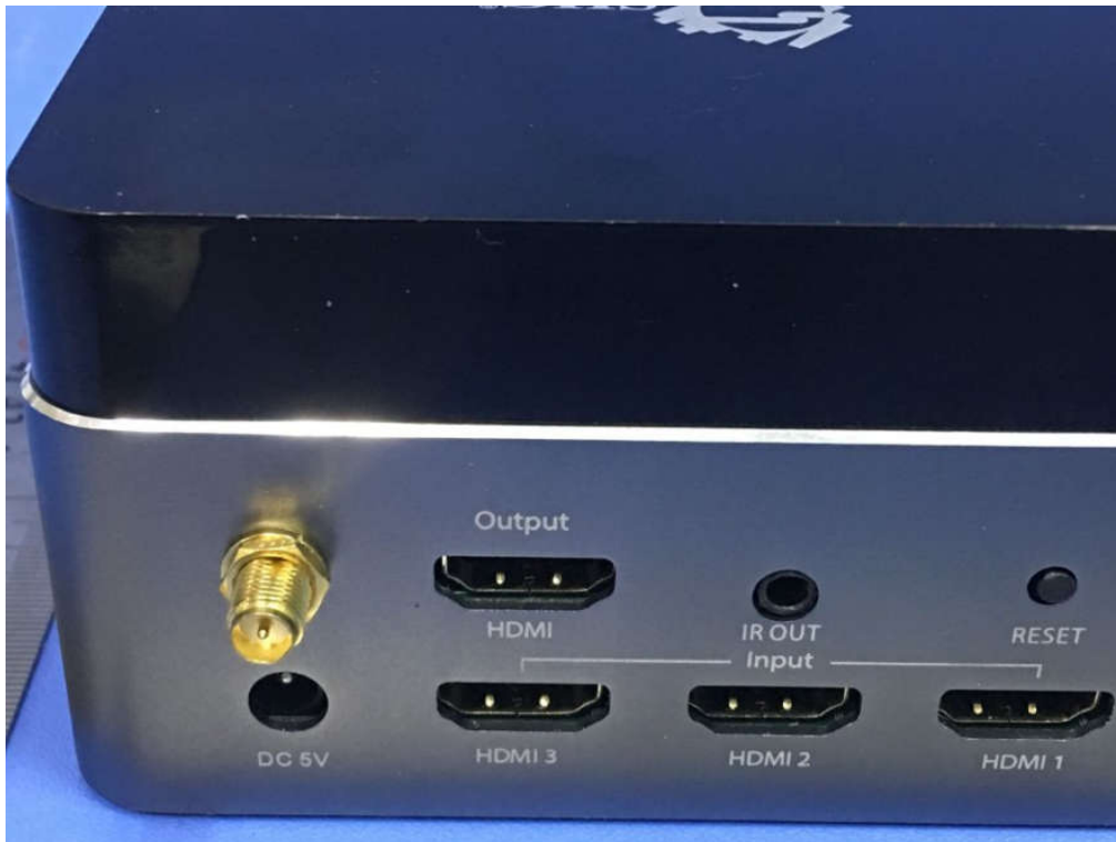
Close view for SMA antenna connector
