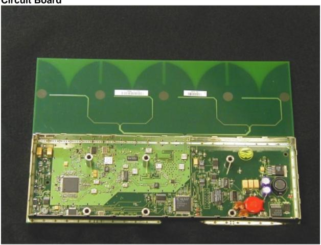
As seen here, the radio is basically a PRISM I chipset with a 1Watt amplifier and a power supply. The FPGA controls the radio via the digital serial link from the computer.
