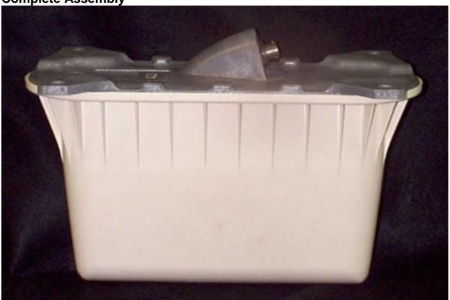
Here is the radio with the plastic cover on. (the internal shield is on the electronics also)
