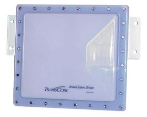
The AA3153 Toll Antenna broadcasts and receives radio frequency signals in the 902 to 928 MHz radio frequency band. It is specifically designed for toll lane applications, with virtually no side or back lobes, which helps confine antenna coverage to a single lane width. The AA3153 Toll Antenna is ideally suited to applications requiring a low profile antenna.
