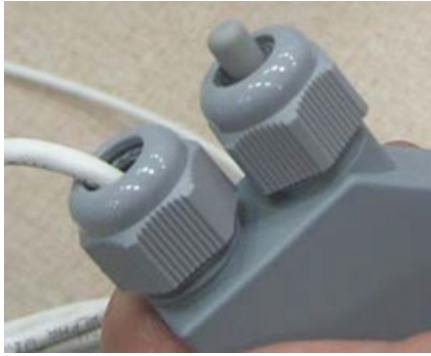
Figure 11–7 Nylon Cap Securely Fastened in Unused Port
