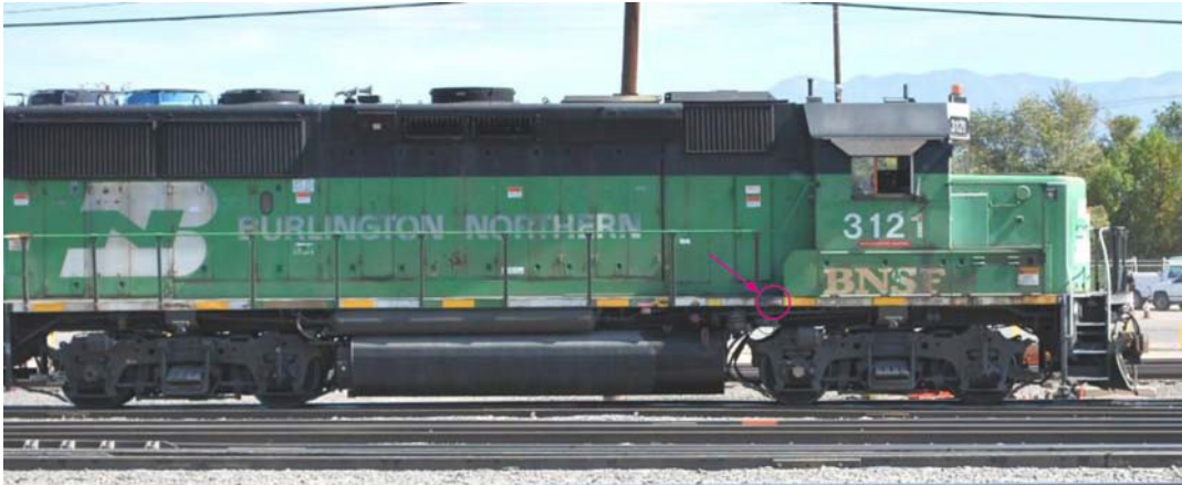
Figure 3–13 Right Front Placement of Tag on Locomotive
