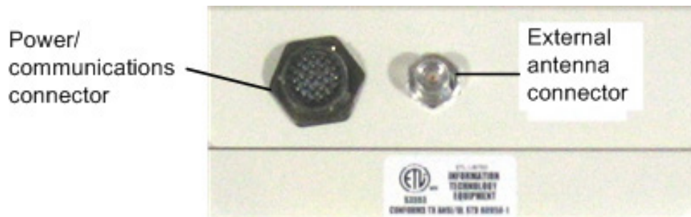
Figure 27 Back of Encompass 4 Reader Showing Antenna Connector
