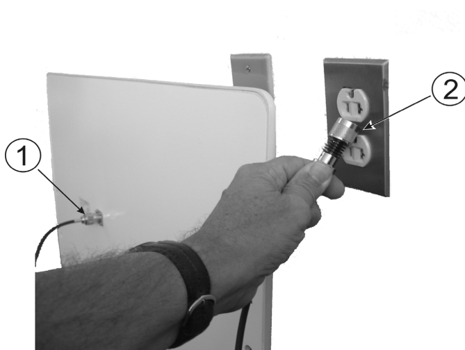
Figure 26 Short Load to Earth Ground
