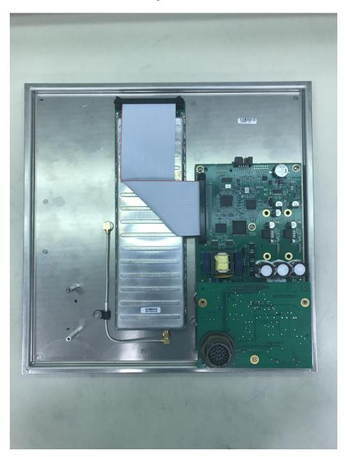
Inside enclosure (back side with power and communications interface board)
