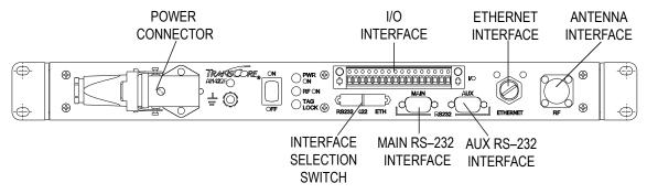
Figure 3 Front Panel of an Al1422E Reader
