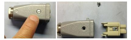
Figure 10 Remove Screw and Plug Insert
