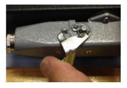
Figure 23 Connector Latch
