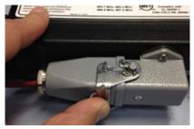
Figure 20 Reinstall Power Connector
