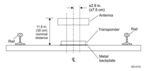
Figure 2 Antenna-to-Tag Centerline Tolerance
