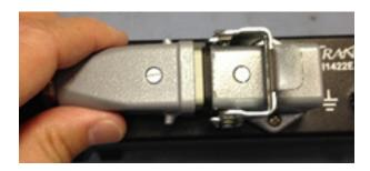
Figure 24 Remove Plug from Receptacle
