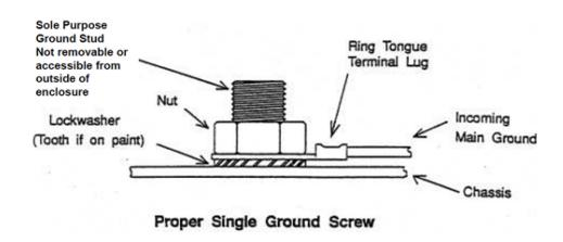
Figure 26 Proper Single Ground Screw Diagram
