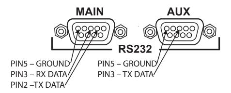
Figure 6 RS-232, DB-9 Interface Connector Pin-outs
