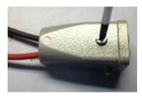
Figure 17 Reassemble and Tighten Set Screw
