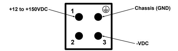
Figure 27 Power Source Connections
