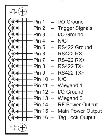
Figure 5 Customer I/O Interface Pin-out
