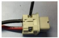
Figure 15 Insert Wires into Pins
