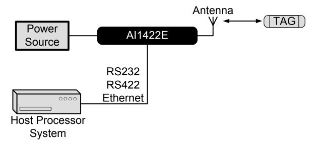
Figure 1 Typical Reader System Configuration
