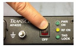
Figure 21 Power the Unit to ON
