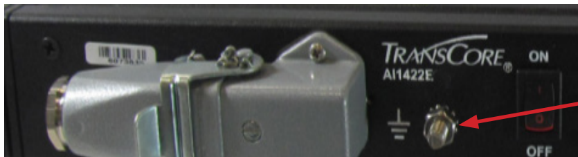
Figure 24 Location of Ground Stud
