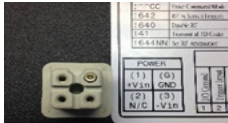
Figure 13 Pin Numbering: Plug Wire Harness
