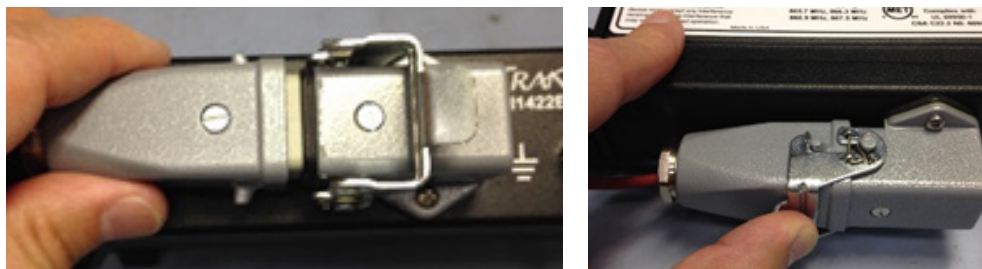
Figure 20 Reinstall Power Connector
