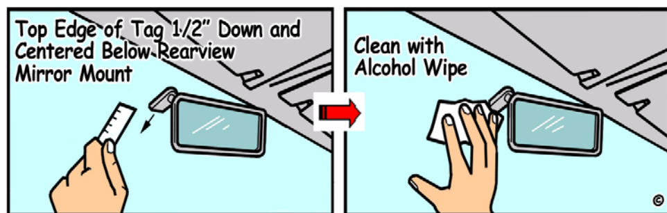
Figure 3-6 eGo Plus Sticker Tag Placement
