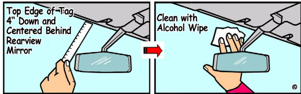
Figure 3-7 eGo Plus Sticker Tag Placement
