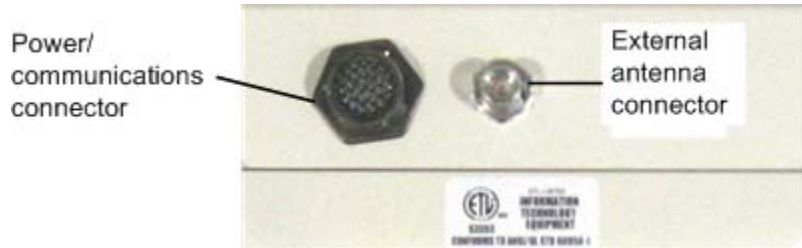
Figure 4-4 Back of Encompass 4 Reader Showing Antenna Connector
