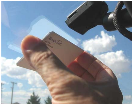
Figure 3-11 Applying eGo Plus Security Sticker Tag to Windshield
