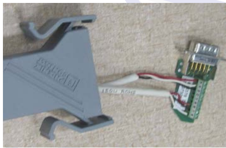
Figure 11-4 Two Check Tag Assemblies Connected to Terminal Strip
