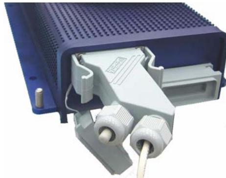
Figure 11-8 Check Tag Assembly Secured to MPRR Port (single check tag assembly shown)
