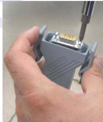
Figure 11-5 Securing Terminal Strip into Connector Housing
