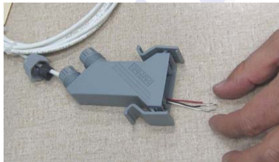
Figure 11-2 Feed Check Tag Wires through Plastic Housing Connector
