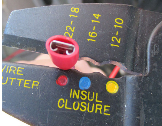
Figure 2 – Crimp Quick Disconnect onto Red Wire
