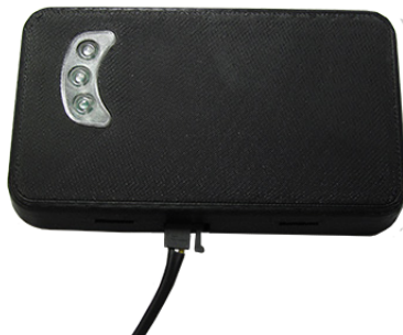
Figure 6 – Connect the Power Cable to the Transponder
