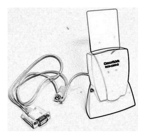
Connect to an available PS/2 connector of your PC. Then connect your PS/2 Mouse/Keyboard to the extension slot at the other side of the connector if necessary.
