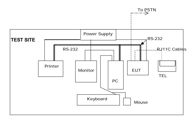
During testing the EUT(External 56K Data/Fax Modem ) was connected to the IBM PC's RS-232 port. So there is no need for additional I/O card. A mouse was connected to the mouse port and a printer was connected to the parallel port. A telephone set was connected to the Phone Jack of EUT and the Line Jack of EUT was connected to a simulator of PSTN.
