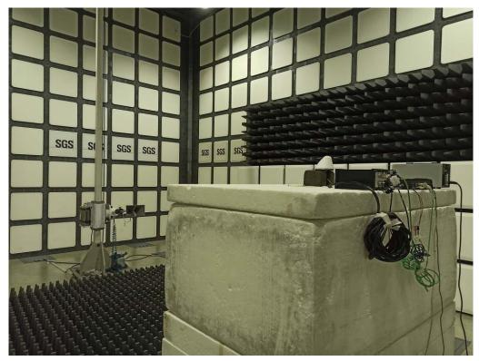
Radiated Emission Set up Photos (Front View)
