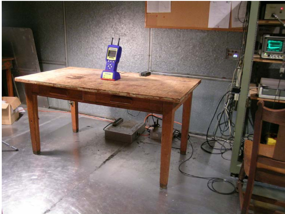
Power Line Conducted Test Setup
