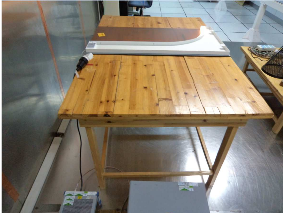
Photograph 1: Set-up for measurement of conducted emission
