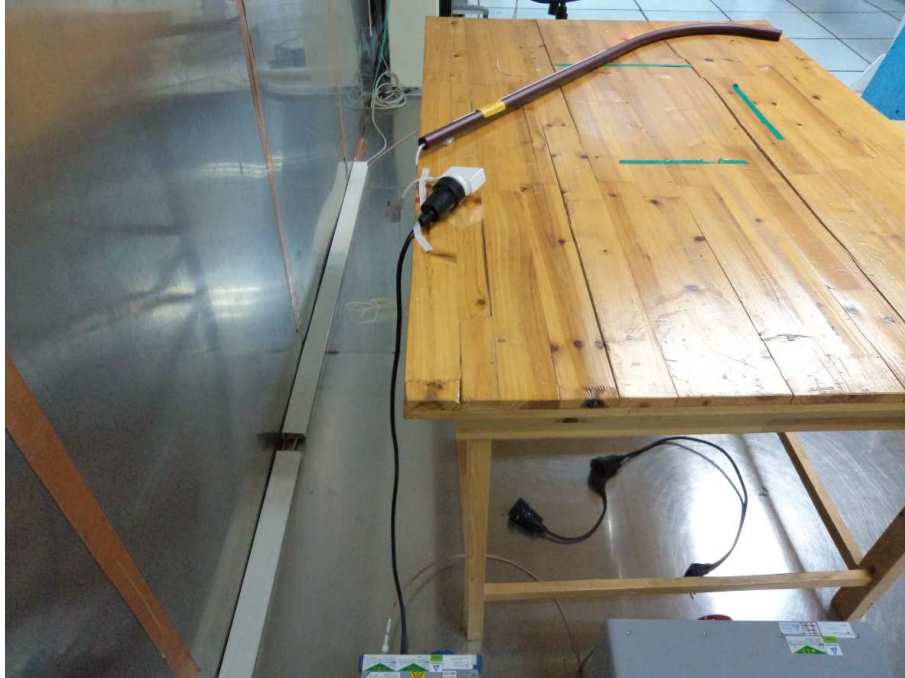
Photograph 1: Set-up for measurement of conducted emission
