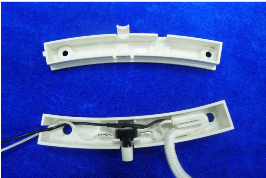
Open view of switch box
