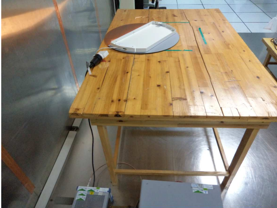
Photograph 1: Set-up for measurement of conducted emission
