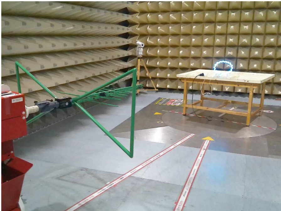
Photograph 2: Set-up for measurement of radiated emission
