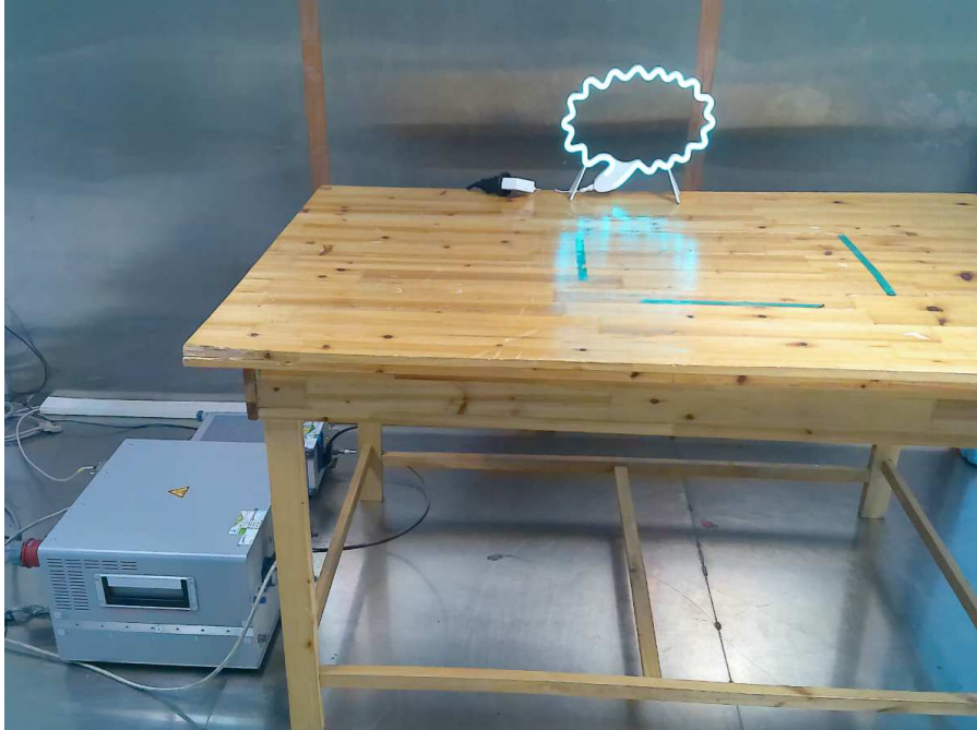
Photograph 2: Set-up for measurement of radiated emission
