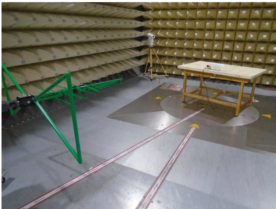
Photograph 2: Set-up for measurement of radiated emission
