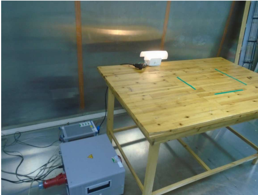
Photograph 2: Set-up for measurement of radiated emission
