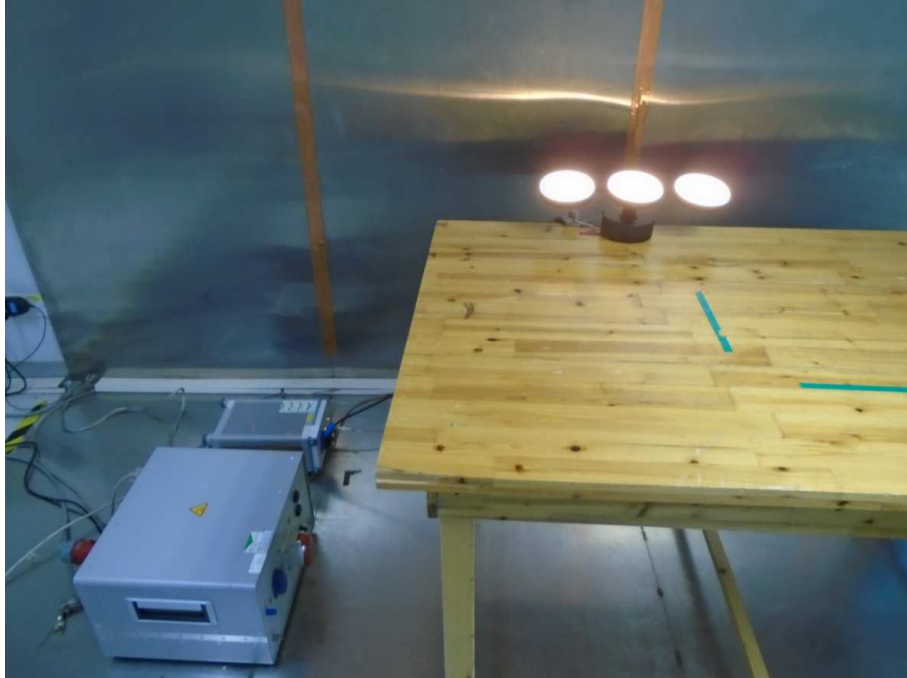
Photograph 1: Set-up for measurement of conducted emission
