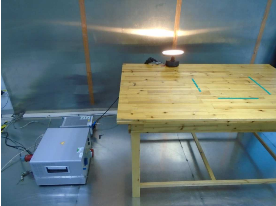
Photograph 1: Set-up for measurement of conducted emission
