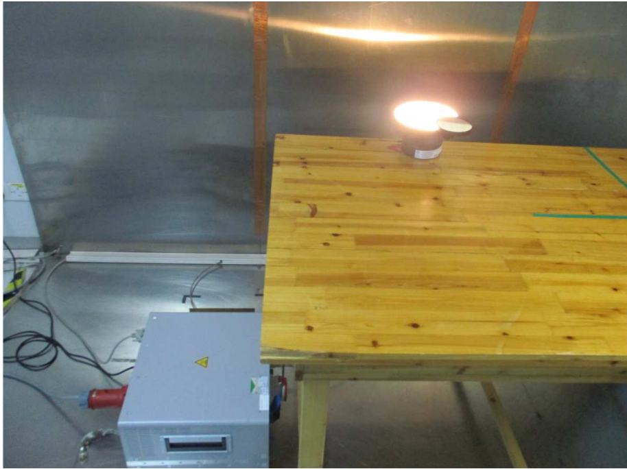
Photograph 2: Set-up for measurement of radiated emission
