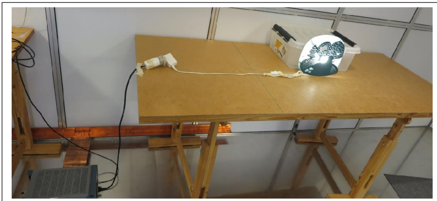
Test setup for conducted emission 150 kHz – 30 MHz
