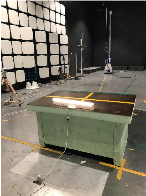
Test set up radiated emission 30 MHz – 1 GHz
