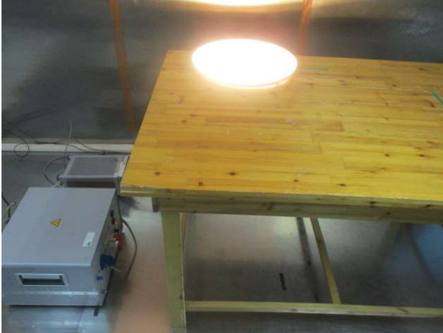
Photograph 1: Set-up for measurement of conducted emission
