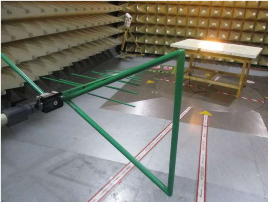
Photograph 2: Set-up for measurement of radiated emission
