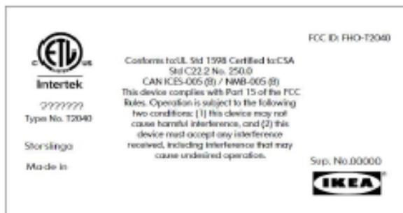
Note: This label was attached on the canopy. The control number "???????" refers to ATM and shall be at least 2mm high.
