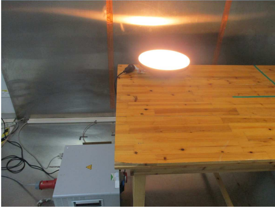
Photograph 2: Set-up for measurement of radiated emission
