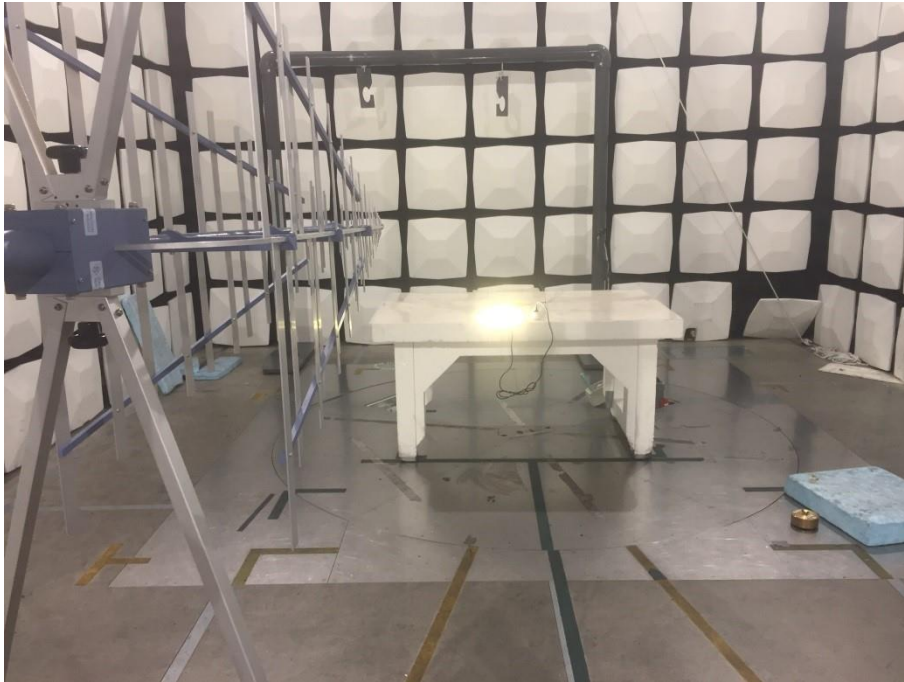
Test set up radiated emission 30 MHz – 1 GHz
