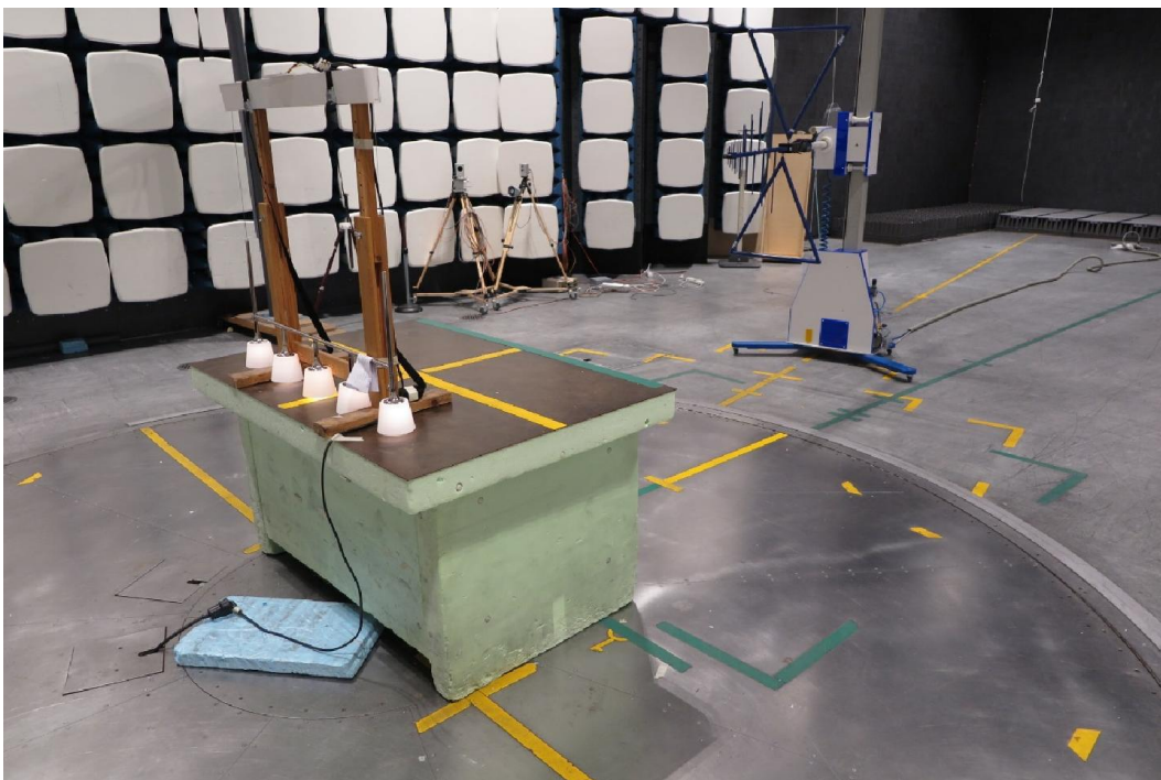
Test set up radiated emission 30 MHz – 1 GHz
