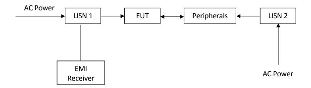
The EUT along with its peripherals were placed on a 1.0m(W)×1.5m(L) and 0.8m in height wooden table and the EUT was adjusted to maintain a 0.4 meter space from a vertical reference plane. The EUT was connected to power mains through a line impedance stabilization network (LISN), which provided 50 ohm coupling impedance for measuring instrument and the chassis ground was bounded to the horizontal ground plane of shielded room. The excess power cable between the EUT and the LISN was bundled.
