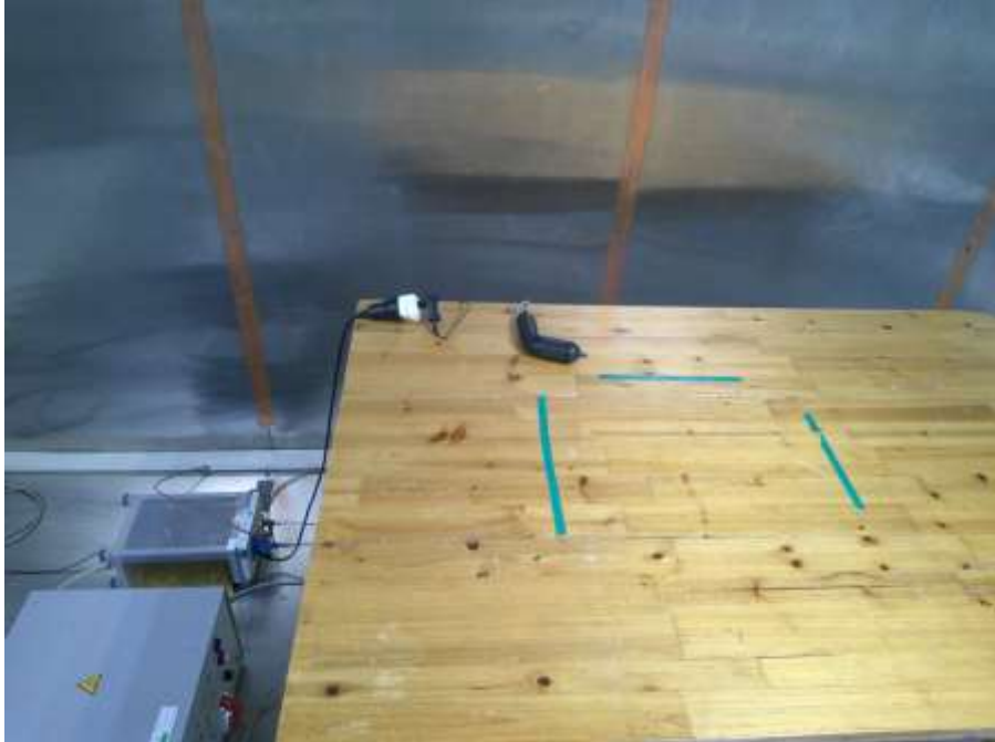
Photograph 1: Set-up for measurement of conducted emission
