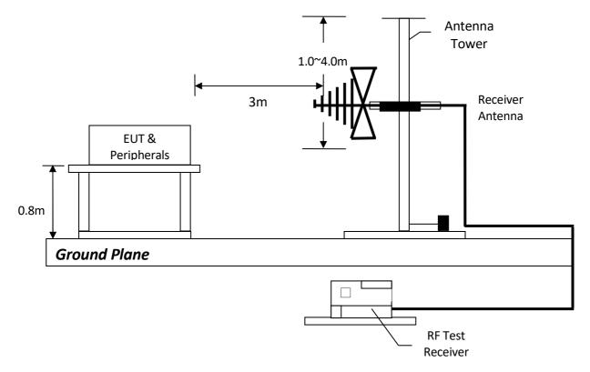
The equipment under test was placed on the top of rotation table 0.8 meter above ground plane.
