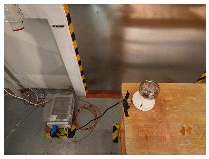
Photograph 2: Set-up for measurement of radiated emission
