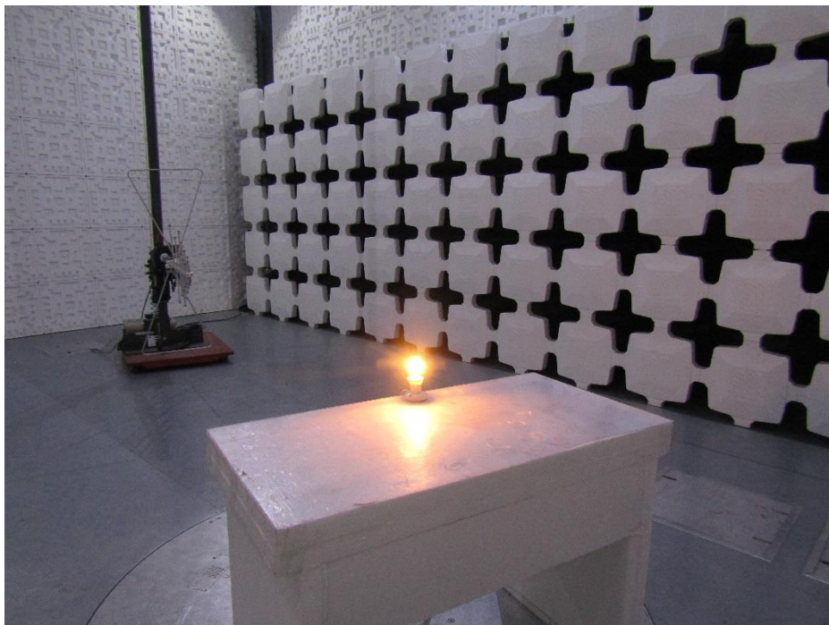
Radiated Emission (30 MHz–1000 MHz)
