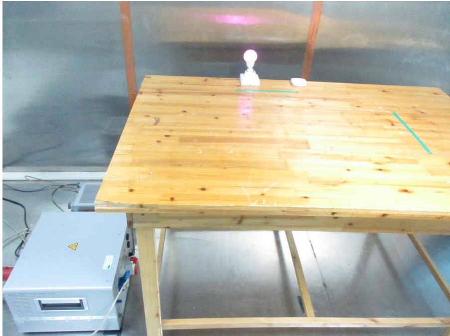
Photograph 1: Set-up for measurement of conducted emission
